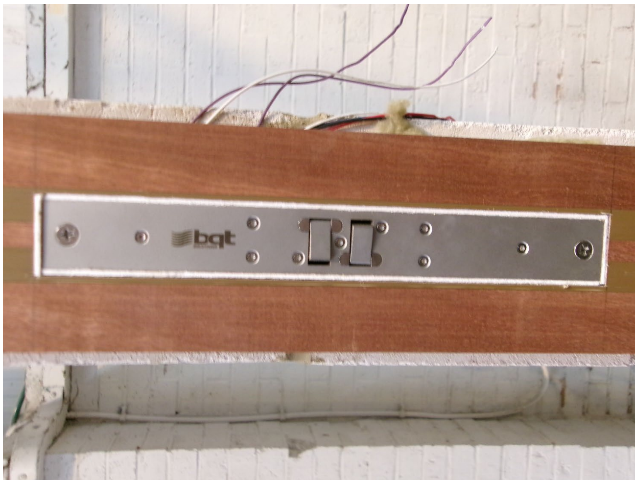
Figure D.5 – Door-Set B – YD30D Leading edge of Frame Pre-Test.
