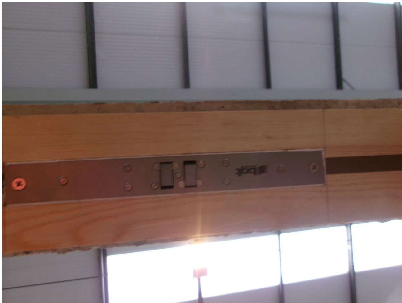
Figure D.4 – Door-Set A – YD30D Frame Header Pre-Test.
